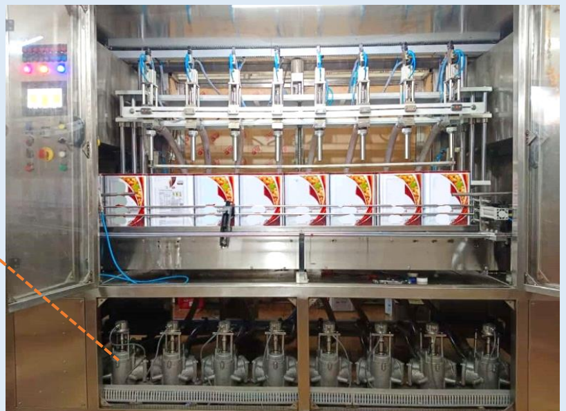
USAGE OF NEOGI METER UNIT IN FILLING MACHINE
